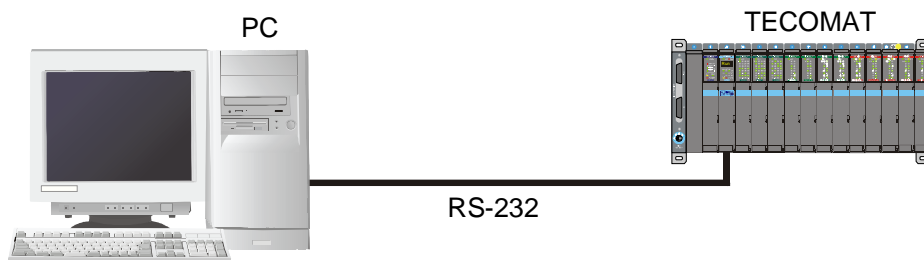
Fig.5.1 Connection to the master system on the RS-232 interface
