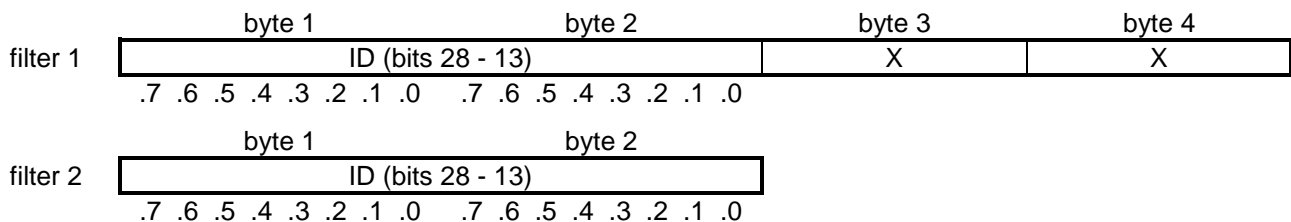
Fig.2.13.6 The structure of the beginning of the received message with the extended frame for the double filter
