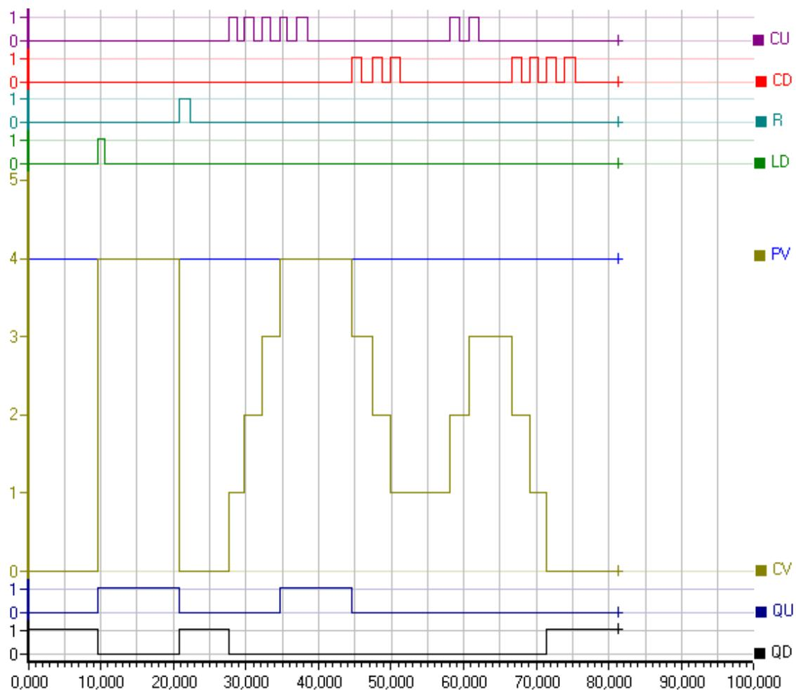
If the value of input variable R is TRUE, the counter value CV is set to zero. If the value of input variable LD is TRUE, then the counter value CV is set to preset value PV.
