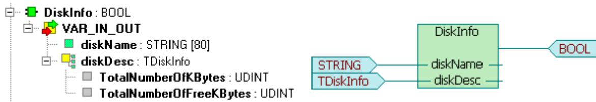
The **DiskInfo** function finds the overall disc size and free space on the disc. The disc name must be stated in the variable *diskName*. If this variable is empty, the **DiskInfo** function restores information about disc that is set as a default disc (e. g. it is a memory card within Foxtrot systems).
