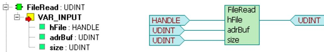
The **FileRead** function load a certain number of characters and save them to the PLC memory. The file is specified by the *hFile* variable. The variable, where the loaded data will be saved to, is specified in *adrBuf*. And finally, the *size* variable states how many characters will be read from the file.
