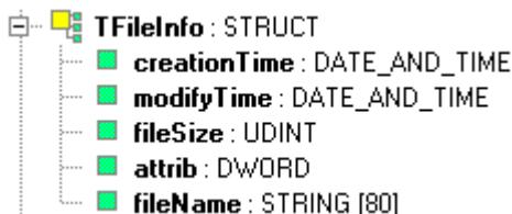
Meaning of individual items of the *TFileInfo* structure is as follows:
