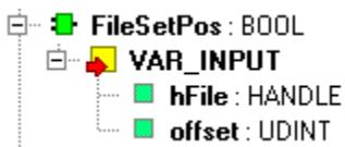
The **FileSetPos** function enables to set the position for the file reading or writing for the file entry. The file is specified by the variable *hFile*. The required position in the file is stated by the variable *offset*.
