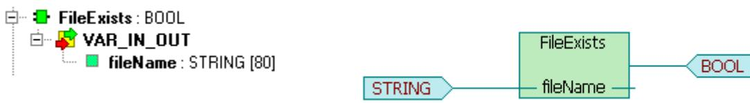
The **FileExists** function tests if the file specified by the *fileName* variable exists.
