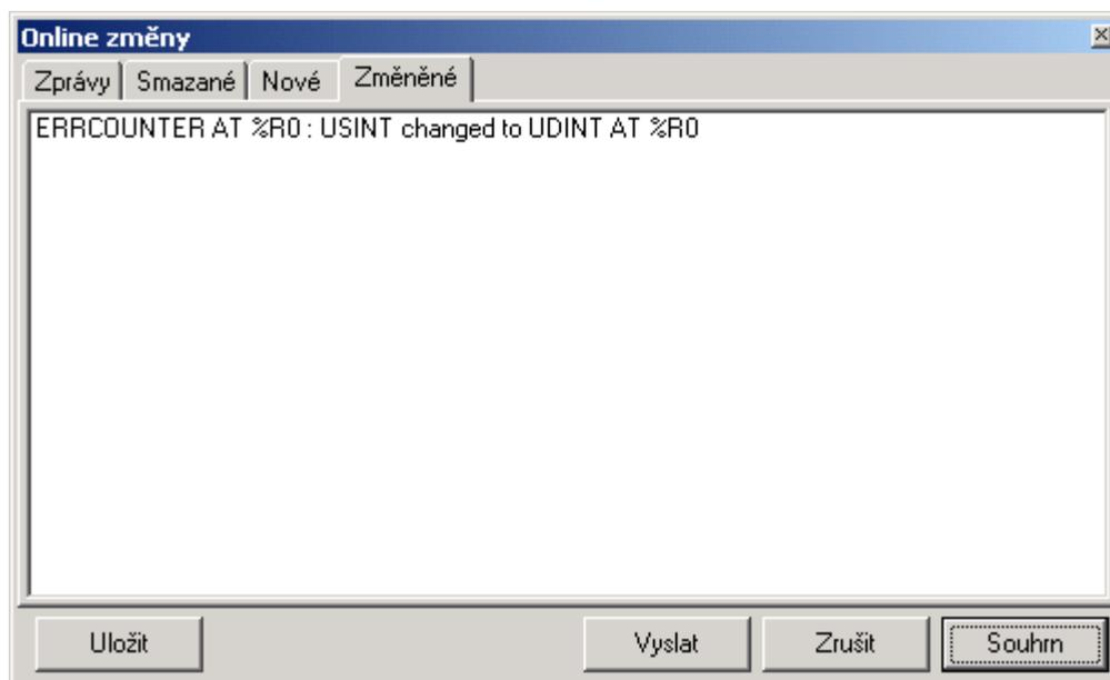
Described changes are undertaken automatically by the PLC central unit in cooperation with the Mosaic environment after the program code is sent from Mosaic to the PLC. Variable values remain the same independently of whether their data type or memory location was changed.
