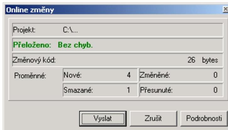
From this dialogue, it is apparent that this change added to the program the total of 4 new variables and one variable from the original program was deleted. This can, on the first sight, seem illogical because we did not delete any variable from the program and we added only two new variables *errCounter* and *tmp*. The explanation can be found in details.
