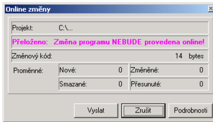
If we choose „Send“, the program code will be send in a standard way because it is a new program. It means that the central unit will transfer to the HALT mode (where outputs are typically blocked), new program will be loaded, restart will be done and then the central unit will transfer to the RUN mode.
