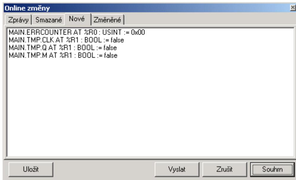
From this window, it is apparent that to the variable *errCounter* corresponds really one new variable while under the variable *tmp* there are hidden three variables really because it is an instance of the function block of the type *R\_TRIG*. Each instance of this function block will then contain variables *CLK*, *Q* and *M* of *BOOL* type.
