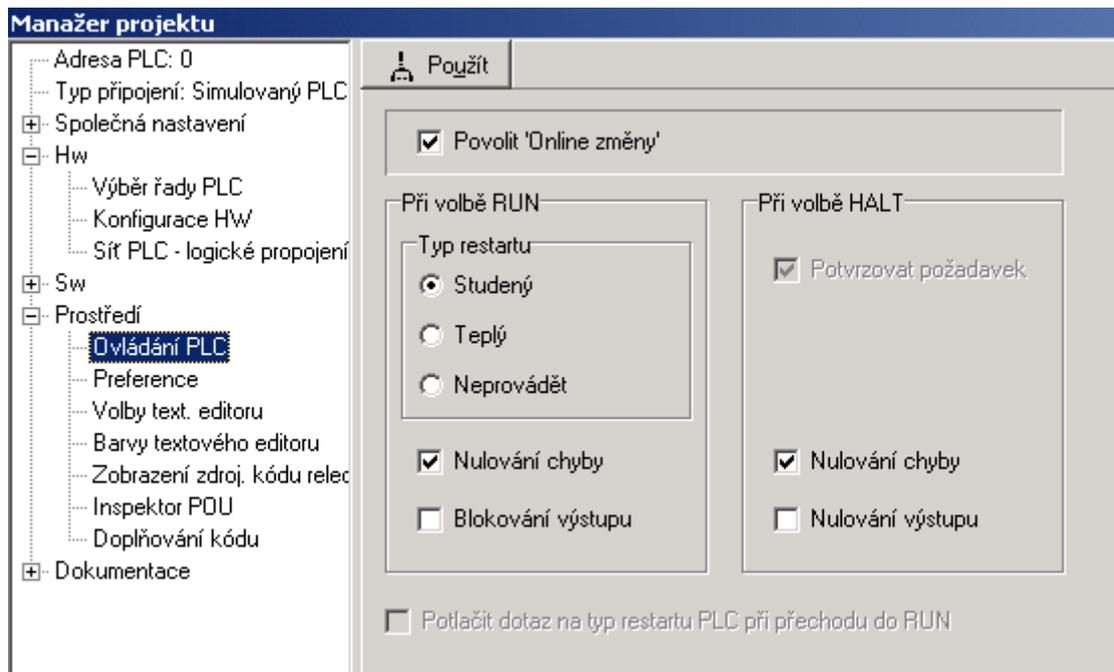
If the PLC central unit does not support on-line changes, the item enabling on-line changes will be grey and the thicking box will not be active.
