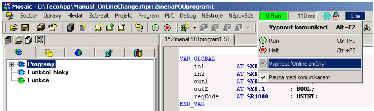
Similarly to the previous description the on-line change can be switched on only in case when the central unit of the PLC support these changes. In other cases the option is not active (grey) and can not be selected.
