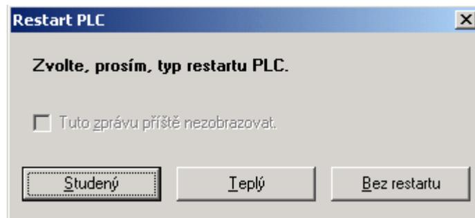
After the restart option is selected, the central unit transfer to the RUN mode. From this moment it is possible to edit the program without control cessation (thus on-line).
