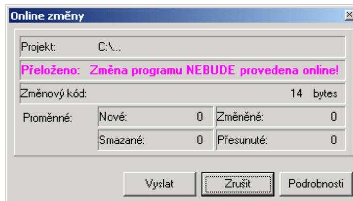
If we choose „Send“ the program code will be sent in a standard way because it is a new program. This means that the central unit transfer to the HALT mode (where outputs are blocked standardly), the new program will load, restart is undertaken and then the central unit transfer to the RUN mode.
