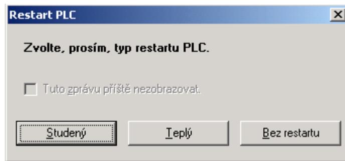
After the selection of the restart type, the central unit transfers to the RUN mode. From this moment it is possible to modify program without control stopping (thus on-line).
