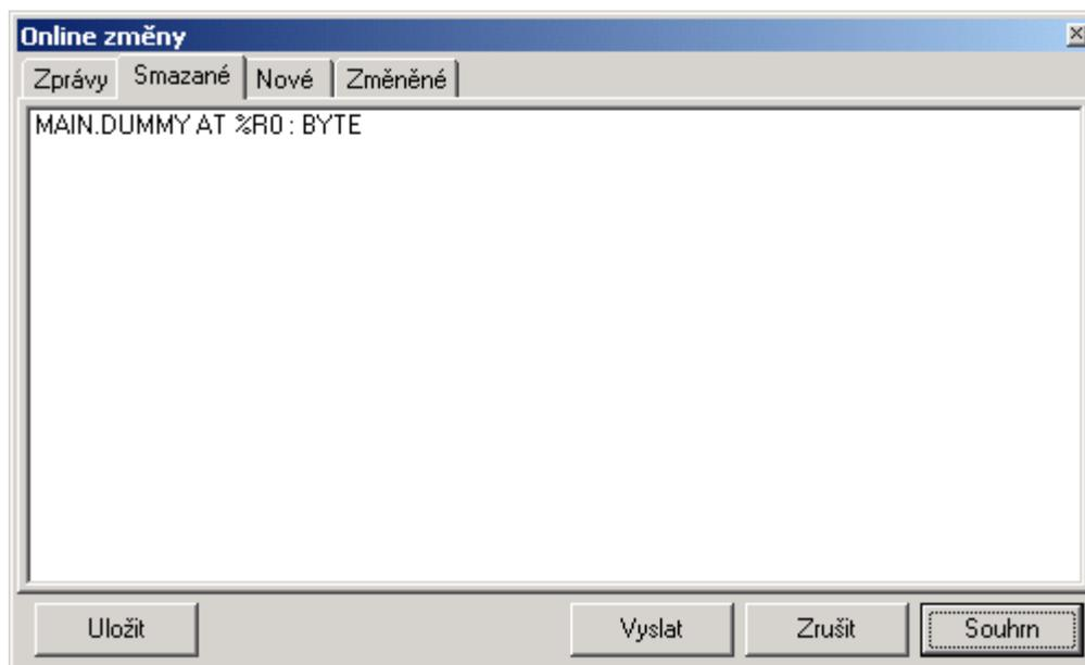
If the POU program has not any local variable declared, the compiler in the Mosaic environment set up automatically at least one empty variable *DUMMY*. In the moment when we add to the program at least one own variable, the variable *DUMMY* loses its purpose and the compiler deletes it. This explains the question of the deleted variable. The variance in the number of new variables is also explained in the details window.
