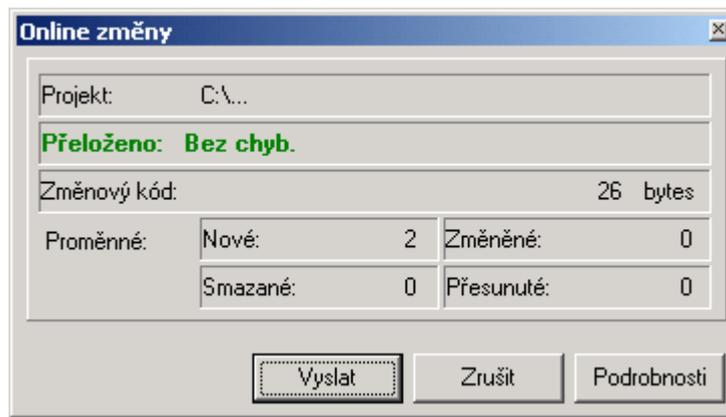
In this dialogue it is apparent that this change added to the program the total of two new variables. These are our variables *errCounter* and *tmp*. We can find out information on this in details.
