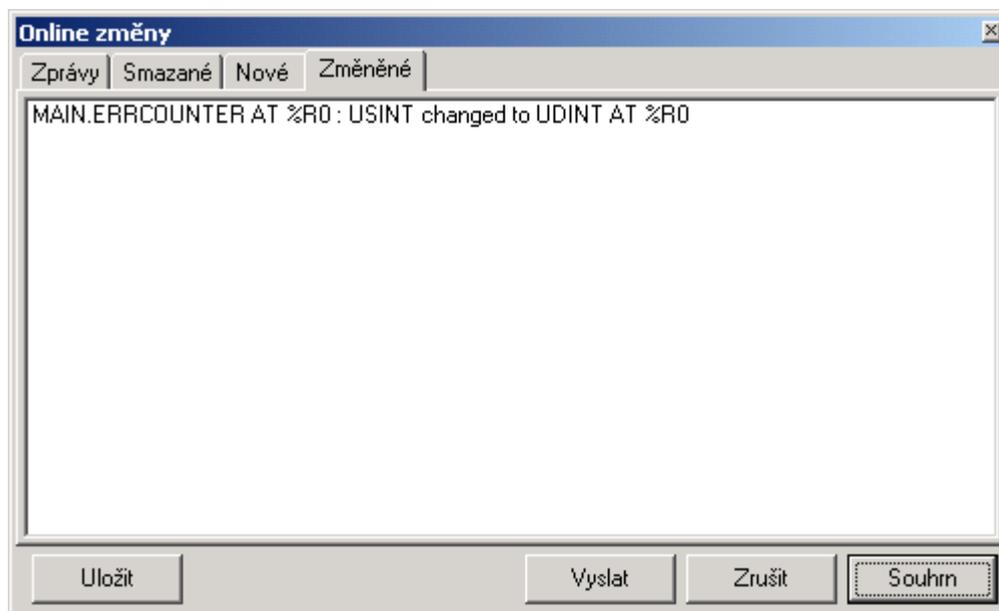
Described changes are managed automatically by central unit of the PLC in cooperation with the Mosaic environment after the program code is sent from Mosaic to PLC. Variables simply keep values independently of changes of their data type or memory location.
