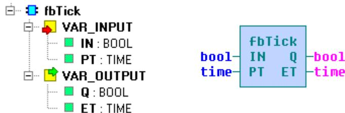
The function block *fbTick* is a timer that generates periodically pulses for the period of one cycle. The input in allows pulse generating, period of generation pulses is determined by the input PT.
