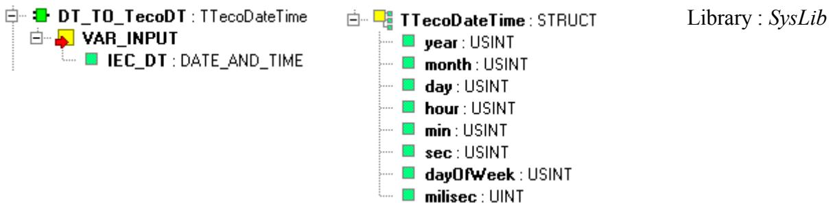
The *DT\_TO\_TecoDT* function transfers date and time from the IEC format **DATE\_AND\_TIME** into the structure **TTecoDateTime**. The advantage of this structure is that there can be operated individually with only some items of time and date as the following example shows.
