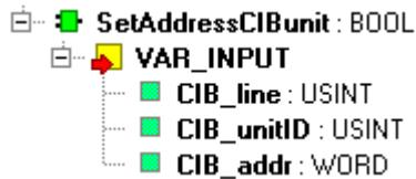
The *SetAddressCIBunit* function sets new HW address of the CIB unit. It can be used in a situation when we want to use similar PLC program for more applications that differ from each other by HW address of CIB units.
