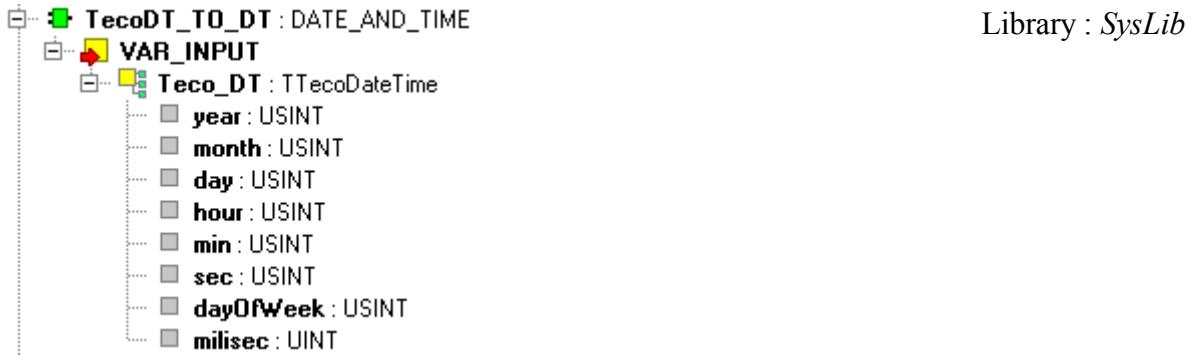
The *TecoDT\_TO\_DT* function transfers date and time from the structure TTecoDateTime to the IEC format DATE\_AND\_TIME.
