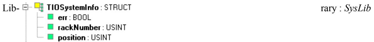
*TIOSystemInfo* type is a structure carrying information about PLC IO system status which is returned by the function *IOSystemInfo*.
