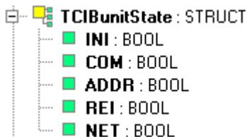
*TCIBunitState* type is a structure carrying information about the status of the unit on the CIB bus which is returned by the function *CIBunitInfo()* as a part of information about the CIB unit.
