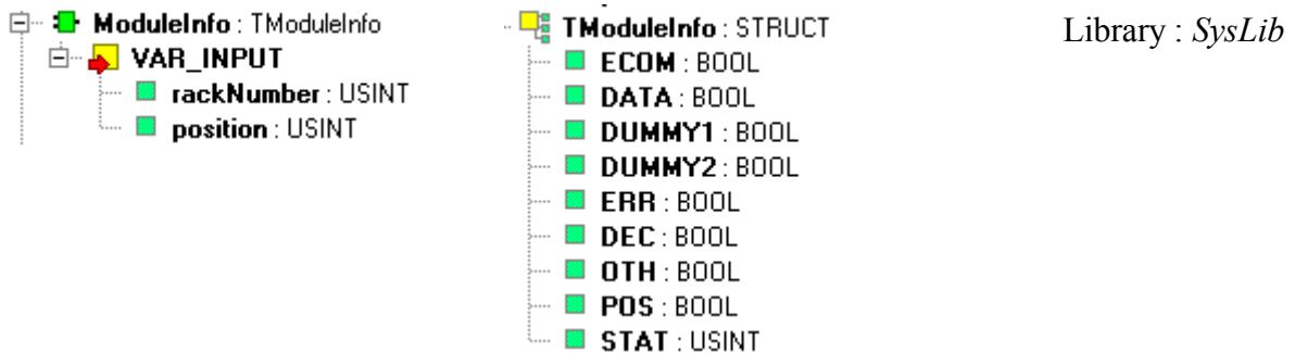
The *ModuleInfo* function returns information about actual status of one I/O module. The input parameter *rackNumber* indicates the rack number and the parameter *position* indicates the position number for which the module information is returned. The function returns the structure *TModuleInfo*.
