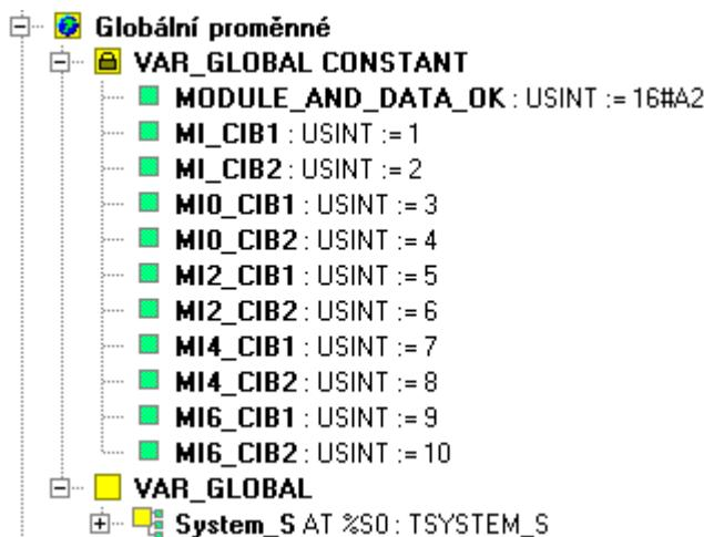
Constants *MI\_CIB1* up to *MI6\_CIB2* are used for specification of CIB line within functions *CIBunitInfo* and *SetAddressCIBunit* and have the following meaning:
