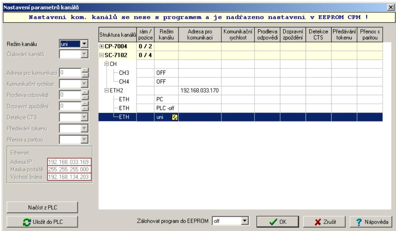
By clicking on the yellow icon on the line ETH uni (highlighted in the previous picture) the next dialogue is initiated where maximum size of sending and receiving zone is set (number of bytes), the type of the TCP slave protocol is selected (PLC will not setup the TCP connection actively) and the port numer is set where data will be awaited (local port).
