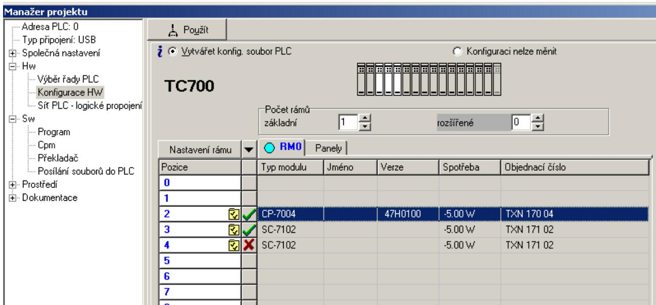
By clicking on the yellow icon on the line with the central unit (here CP-7004), the dialogue for ethernet interface setup is opened. In this dialogue, it is necessary first to switch on the uni mode of the channel on the ethernet interface so, that we click on the line ETH uni-off (highlighted in the following picture) and then we switch the channel mode in the left upper corner from the value OFF to uni.
