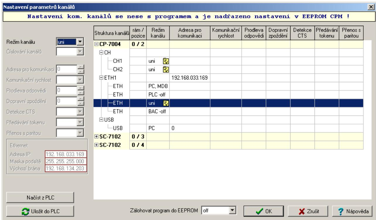
By clicking on the yellow icon on the line ETH uni (highlighted in the previous picture) the next dialogue is initiated where maximum size of sending and receiving zone is set (number of bytes), the type of the TCP master protocol is selected (PLC will setup the TCP connection actively) and the IP address of the system is set where data will be sent to. The remote port is a port where data will be sent to, the local port is, on the contrary, a port where data are sent from.
