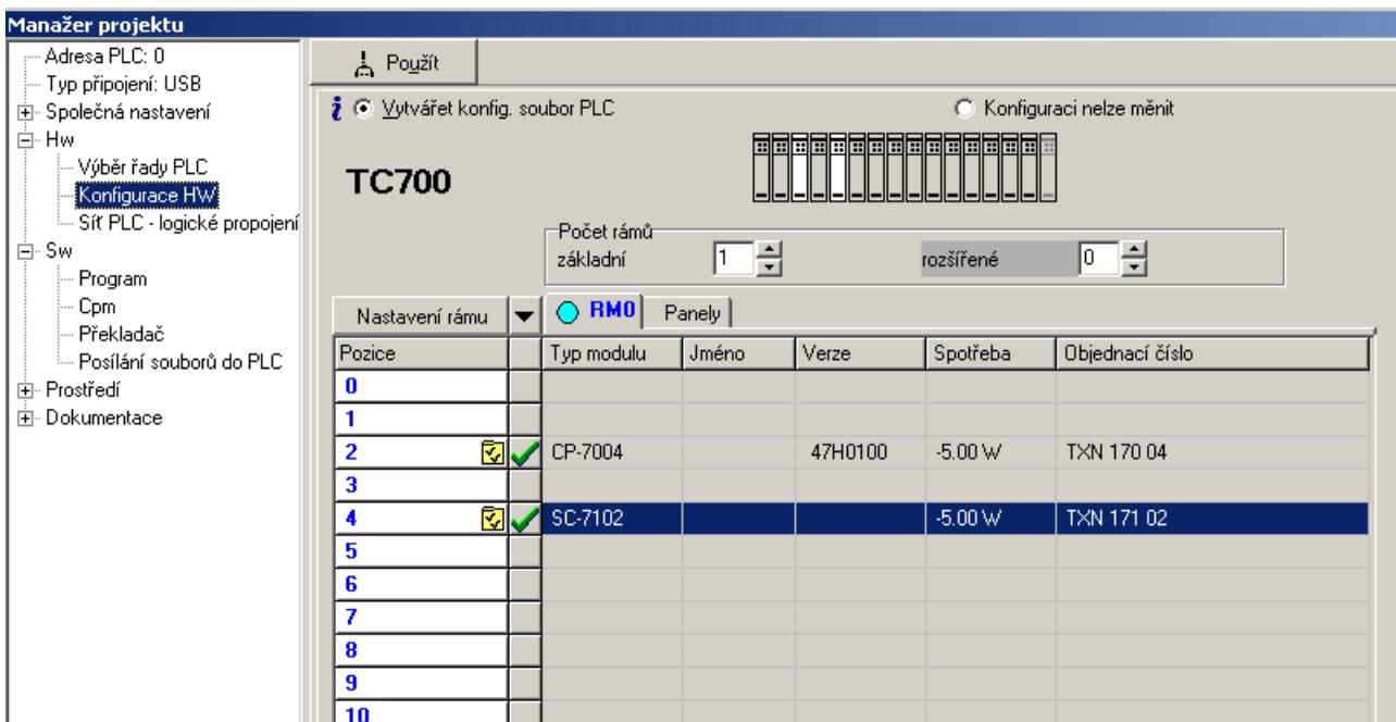
By clicking on the yellow icon of the module SC-7102 (see the highlighted line in the following picture) the setting of communication for module SC-7102 is initiated. In this dialogue, it is necessary first to switch on the uni mode of the channel on the ethernet interface so, that we click on the line ETH uni-off (highlighted in the following picture) and then we switch the channel mode in the left upper corner from the value OFF to uni.
