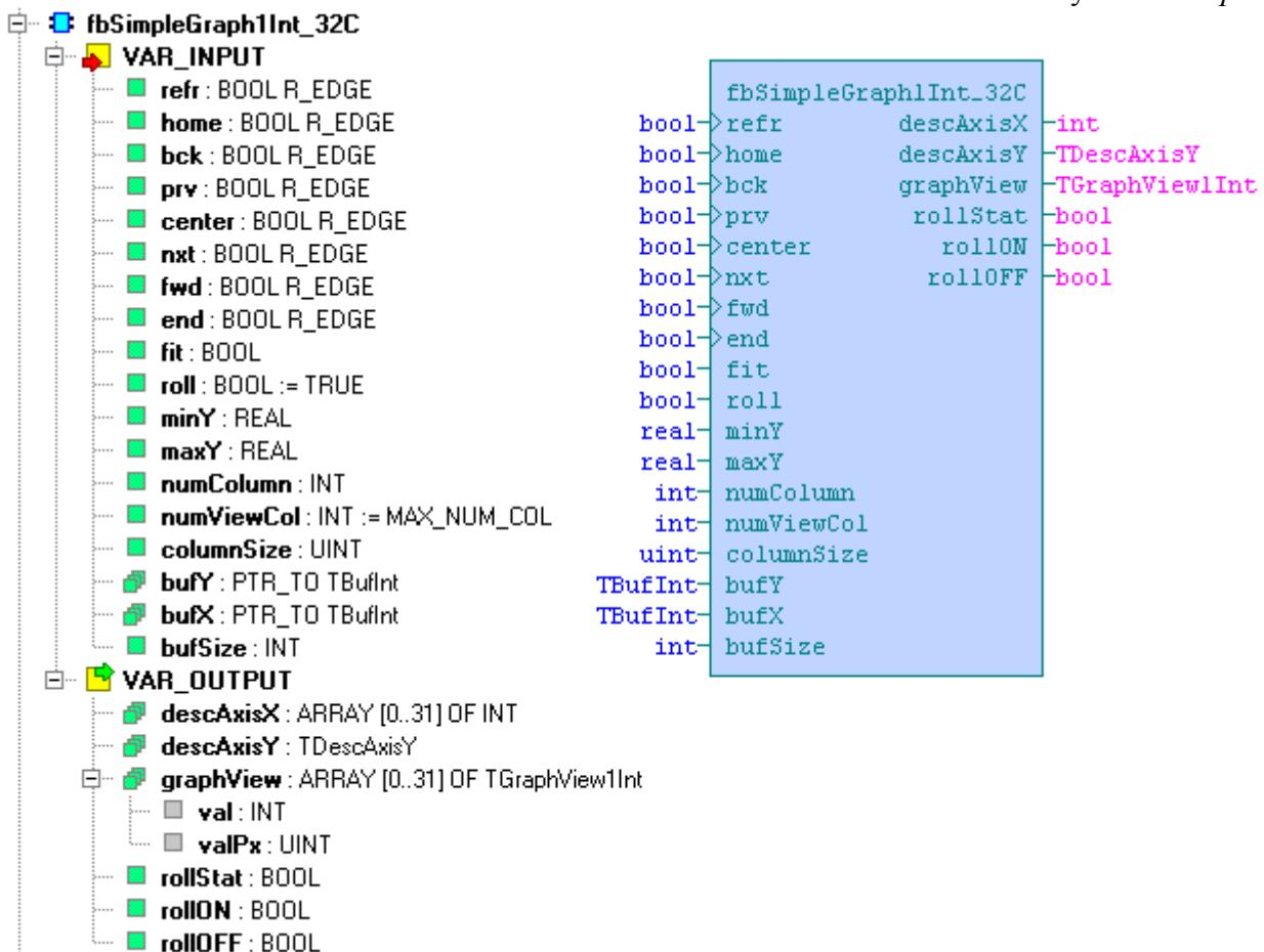
Function block *fbSimpleGraph1Int\_32C* is used as a support for the graph of one variable of the INT type. Maximum number of displayed samples is 32.
