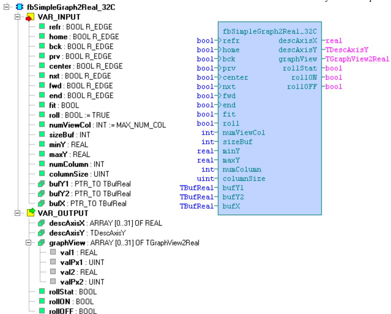
Function block *fbSimpleGraph1Real\_32C* sis used as a support for the graph of two variables of REAL type. Max number of displayed samples is 32.
