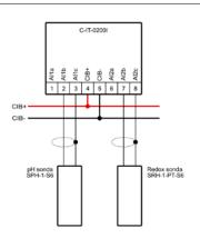
Example of connection pH and Redox probes
